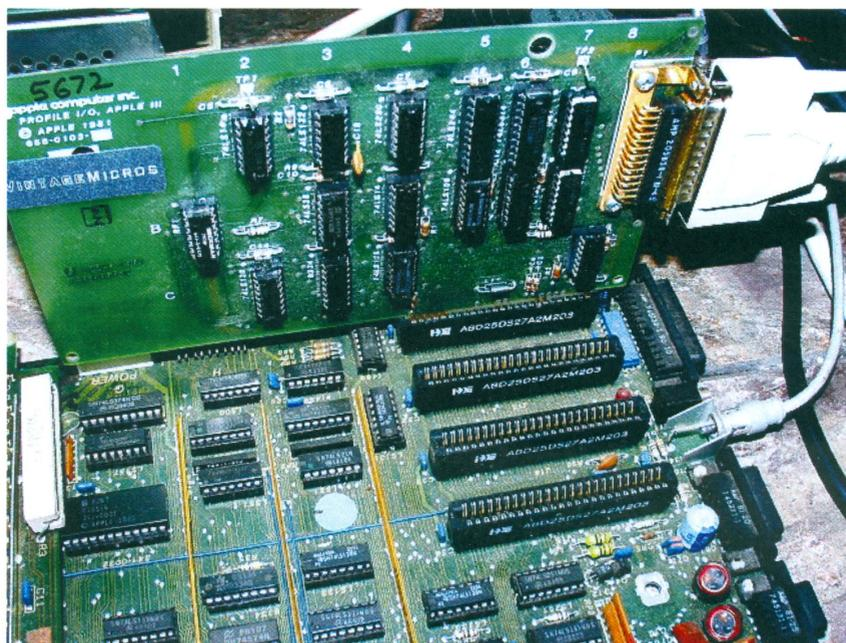
Without turning on the Apple III, connect the cable between the interface card and the Profile. **Do NOT shut down the Profile to do this. Leave it powered up and running.**
